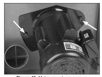
Figure 43. Motor mount cap screws.
